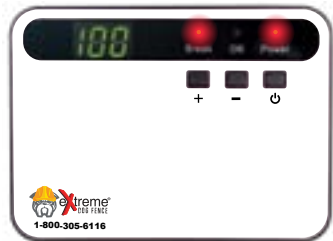
Power On, wire broken or not installed
