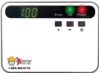
Power On, wire correctly installed and working
